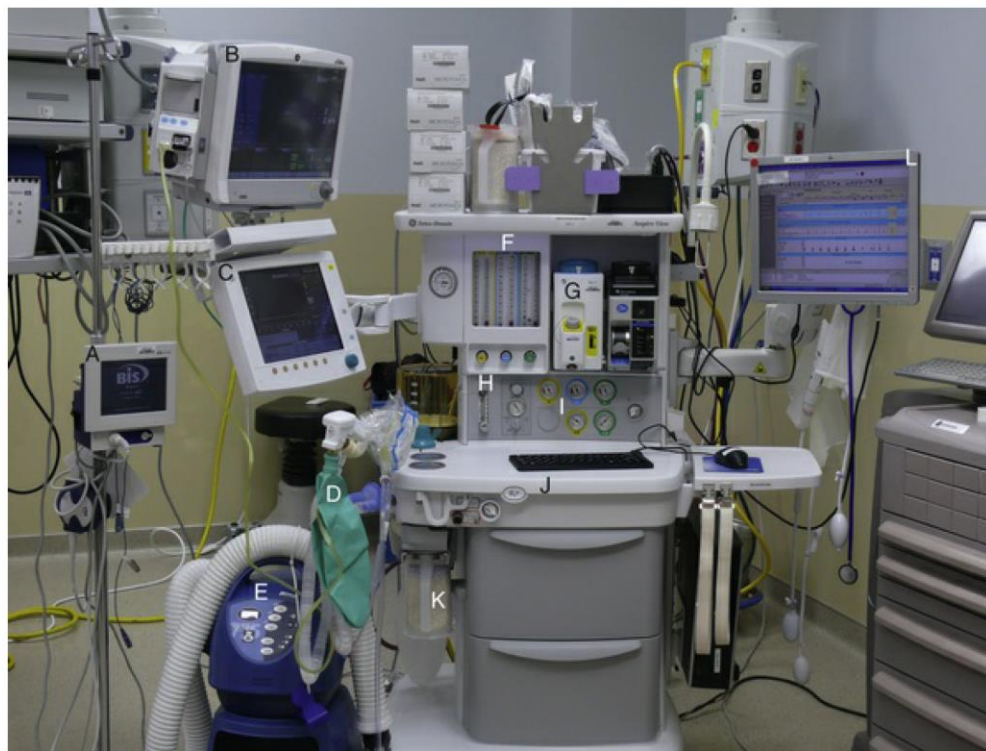
FIG. 5.1 Modern anesthesia machine. (A) Bispectral index system monitor. (B) Patient vital signs display monitor. (C) Ventilator display monitor. (D) Patient breathing circuit. (E) Bair Hugger patient warmer. (F) Gas flowmeters. (G) Anesthetic vaporizers. (H) Supplemental oxygen supply. (I) Oxygen, air, and nitrous oxide gauges. (J) Oxygen flush valve. (K) Carbon dioxide absorber. (L) Electronic recordkeeping screen.
