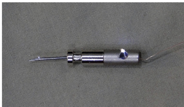
Fig. 1. Probe conducting to cloth over aluminum foil. Note arcing in the wire-probe connection eye.
